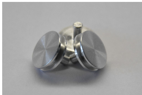
Figure 16 Stubs used for mounting specimens in order to prepare them for an SEM imaging process. Source: http://en.wikipedia.org/wiki/Scanning_electron_microscope
